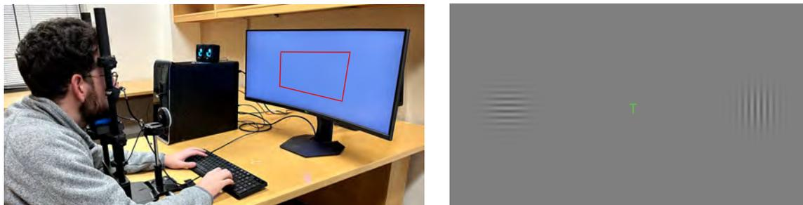
**Figure 4.3:** Our setup for measuring contrast thresholds under differing attention conditions. A photograph of the user study setup is shown on the left. An enlarged illustration of the stimulus on the screen (outlined in red) is shown on the right. The central RSVP letter task with the Gabor wavelets centered at  $e$  to the left and right. The brightness of the letter “T” and the contrasts of the Gabors have been exaggerated for visibility.
